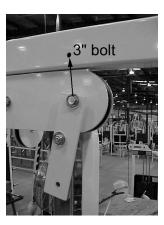
Figure 13. Mount adjustable pulley bracket.
